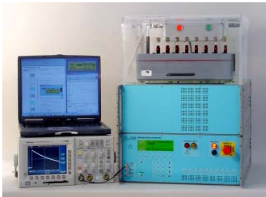
Test set-up with MIG1212CAP and DUT-MUX
