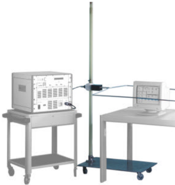
MSURGE 1mx1m antenna mounted on support stand shown with a monitor as EUT (right) and a PSURGE6 as impulse generator (left)
