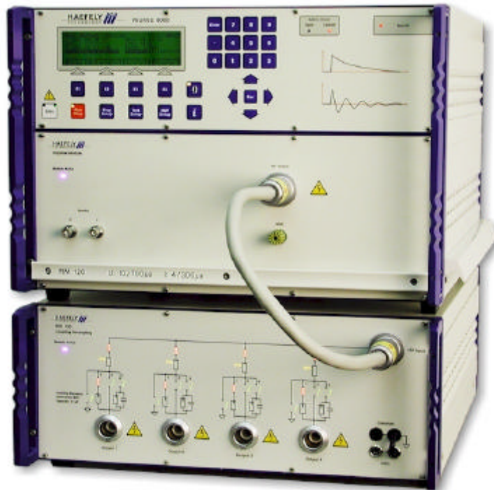
PIM 120 impulse module (upper) with PCD120 coupling network (lower)
