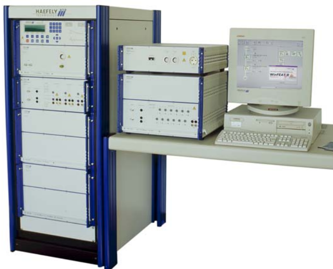
PIM910 impulse module (lower in rack) and controller (PSURGE8000) with user interface and remote control (from PC) using WinFEAT&R software
