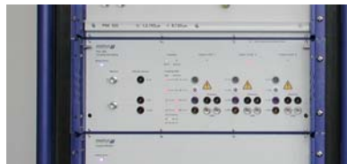
PCD900 coupling module (middle) meets GR-1089 test conditions A & B
